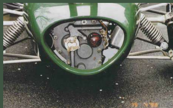
The car came complete with the original Type 32 Colotti 5-speed gearbox as supplied with the car when it was new to Jack Brabham. (Hall & Hall)
