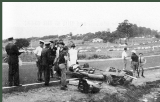
Syd van der Vyver's 24-947 after its Westmead crash. The chassis has been twisted by the impact, which looks to have been at the left rear. The nose has been parted from the rest of the top-body section, with both parts lying in the foreground, while the engine cover also shows signs of the car having rolled. (Graham Vos)
