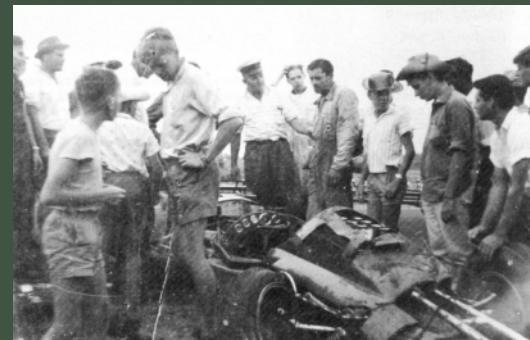
This shot shows more clearly that the upper-left chassis rail between the cockpit and engine bulkheads has been badly bent. A shocked-looking Van der Vyver surveys the wreckage, with a medical officer holding his arm. (Graham Vos)
