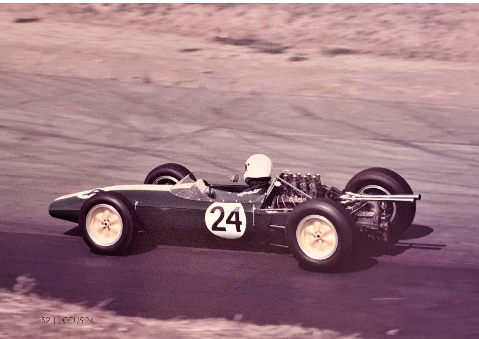
Warren Sankey driving 24-947 in a historic racing event during the first season he raced the car, 1984, at an unknown track. Note the car is still running its original Type 32 Colotti 5-speed gearbox but without an engine or gearbox cover. (Patrick Gearing)
